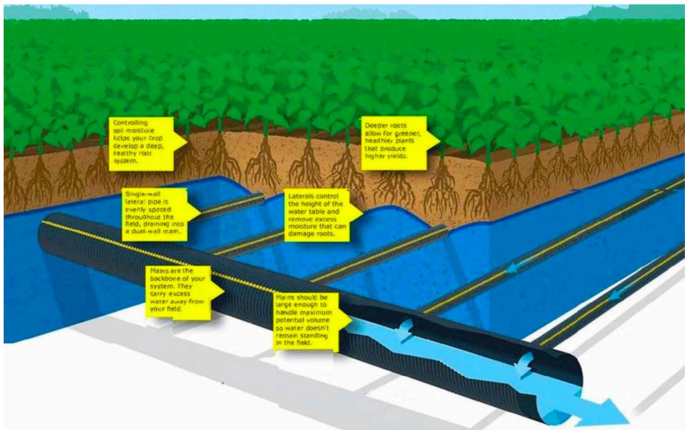
A tile drainage system consists of a network of below ground pipes called laterals and mains that work together to manage the water table. The laterals are spaced throughout the field and collect water that travels to a main. The main allows the system to carry the water out of the field in a controlled and responsible fashion. An entire drainage system is designed on a grade (or slope) so the water flows in a specific direction.
